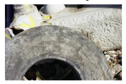
Goodyear aircraft tire. The "spare" seen behind is aircraft landing gear sections.
