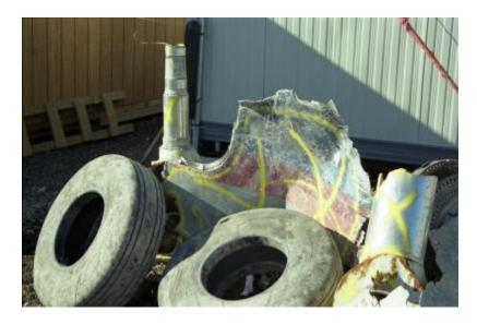
Detail of airplane landing gear, tires and fuselage fragments.
