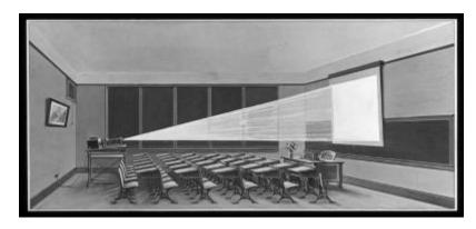
A drawing of a room fitted for use of projection lantern, including arrangement of shades for darkening the room, the lantern on a movable stand, the baseboard electric outlet, and the screen attached to picture molding.
