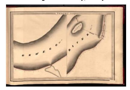
This is an ink, wash and charcoal map of a section of the Oswego Canal in Volney. The map shows the Oswego River, an unnamed island, two dams, and two bridges. The red lines indicate courses and distances. The blue lines indicate canal right-of-way.
